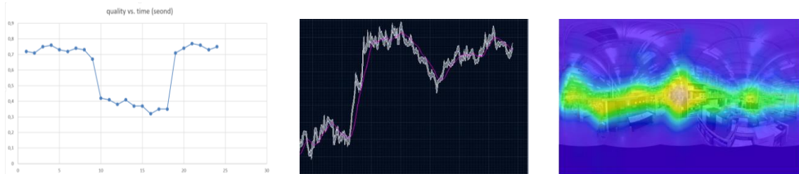
Figure 26: Graphical representation of the output data. a) Video quality changes in time b) Moving averaged delay which shows the trend of delay changes (red line) c) Fixation map shows the locations focused by users.
