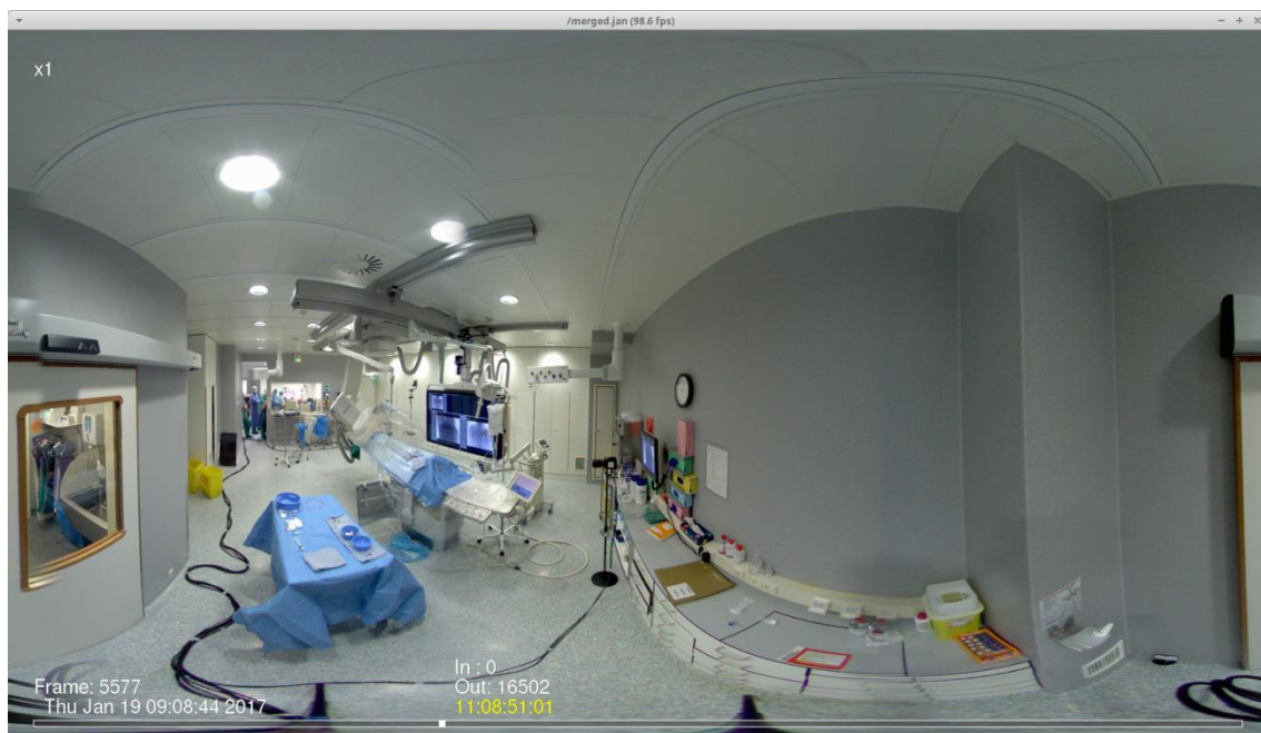
Figure 24: Equirectangular video produced simultaneously with previous. (In fact, a semi-omnidirectional camera would have been better for this point of view, as the action is concentrated in less than 170 degrees field of view.)
