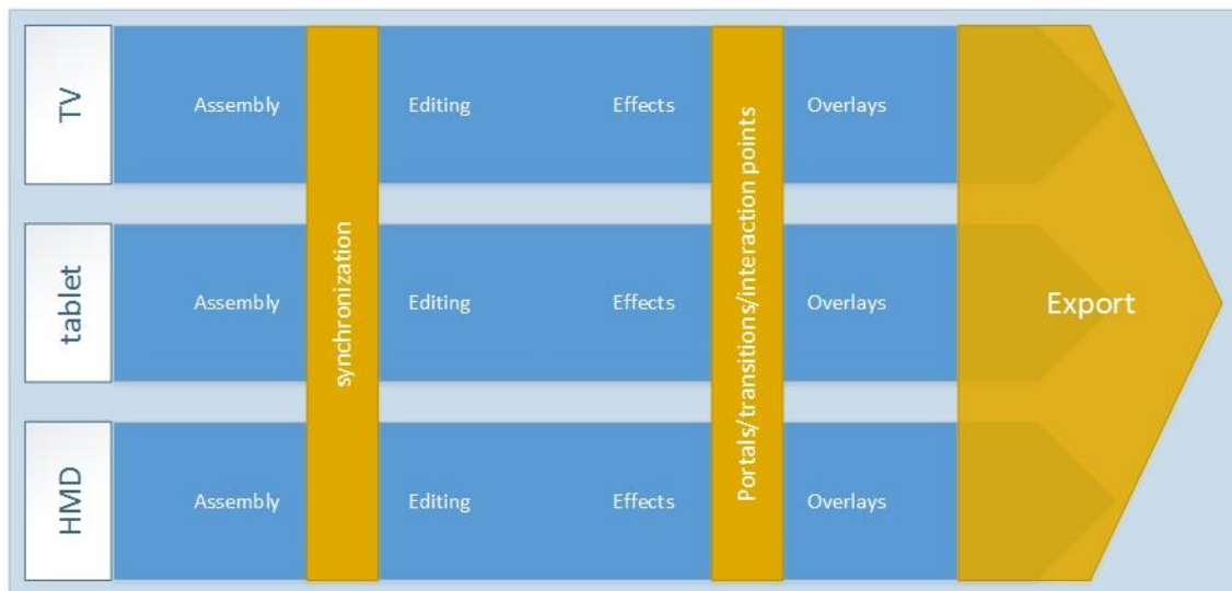
Figure 8: Schema of proposed editor workflow
