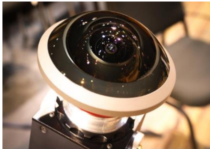
Figure 34: AZiLPix Studio.One single-lens VR video capture solution, utilizing an extreme fish eye lens covering 5/6 th of the full sphere in a single (absolutely seamless) video.
