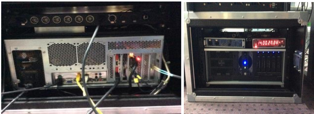
Figure 22: Studio.One server in rack mount case with time code generator and audio interface and robust connectors to stage box, cameras and control room.
